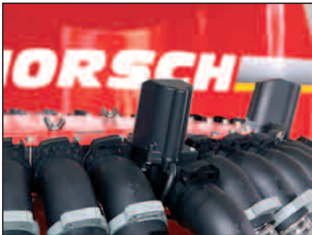
Motorised valves for tramline control
