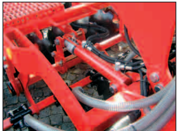
Adjusting the working depth of the fertiliser coulters
