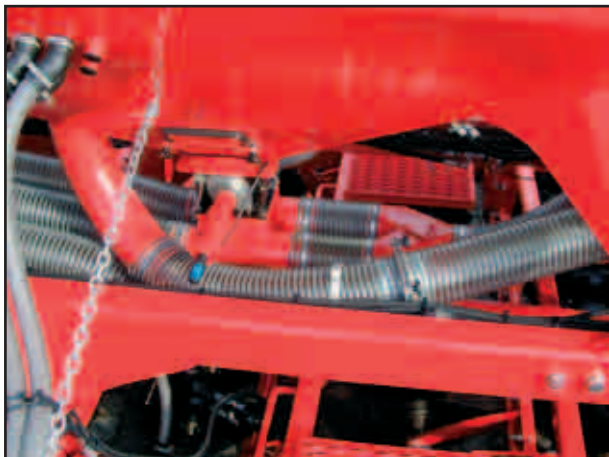
Fan hose connection and seed hose
