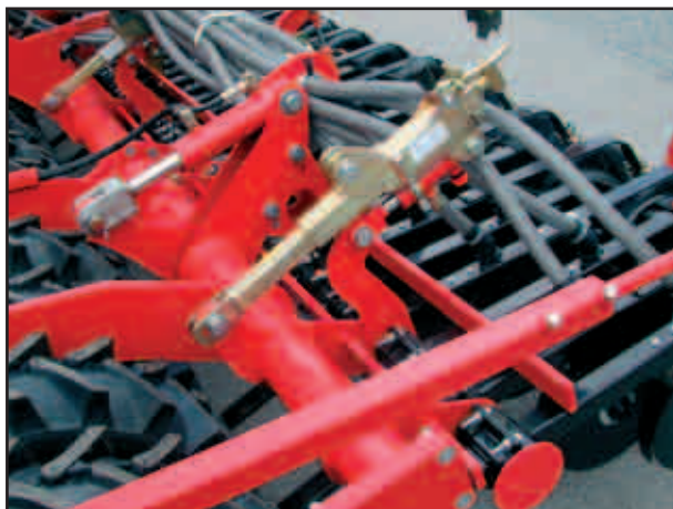
Hydraulic coulters pressure adjustment
