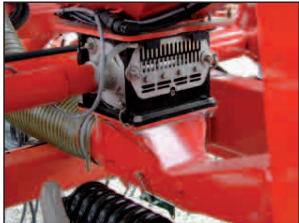
Metering unit with cover for injector nozzle
