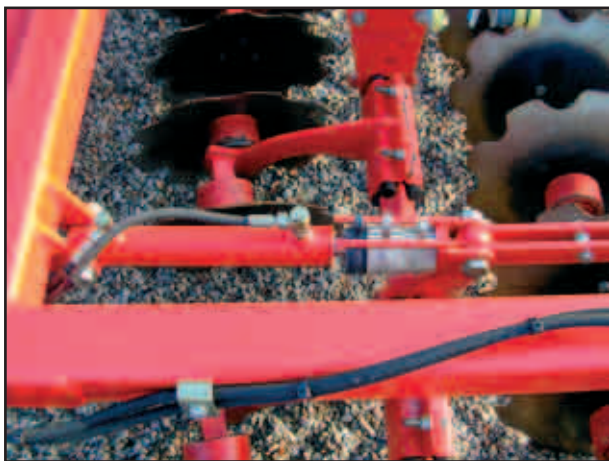
Hydraulic cylinder depth setting with aluminium clips
