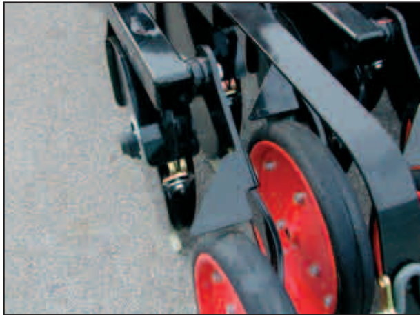
Scraper for coulters discs and press wheels
