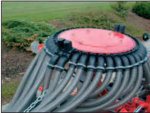
Seed distribution box with motorised valves for tramline control
