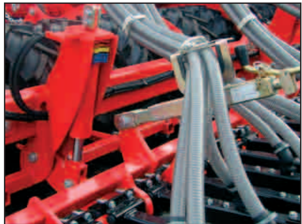
Hydraulic cylinder and adjustment crank handle
