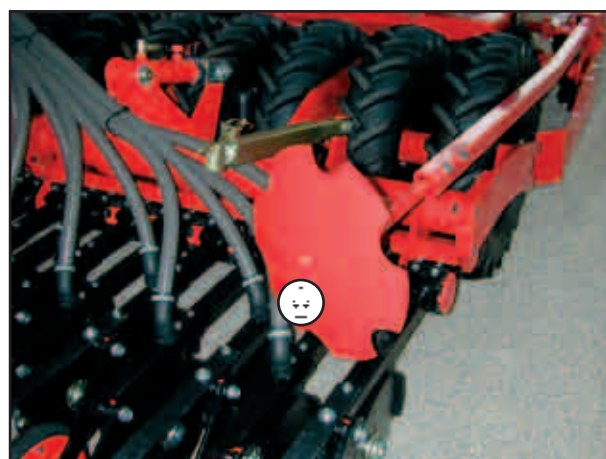
Lubricate the bout marker
